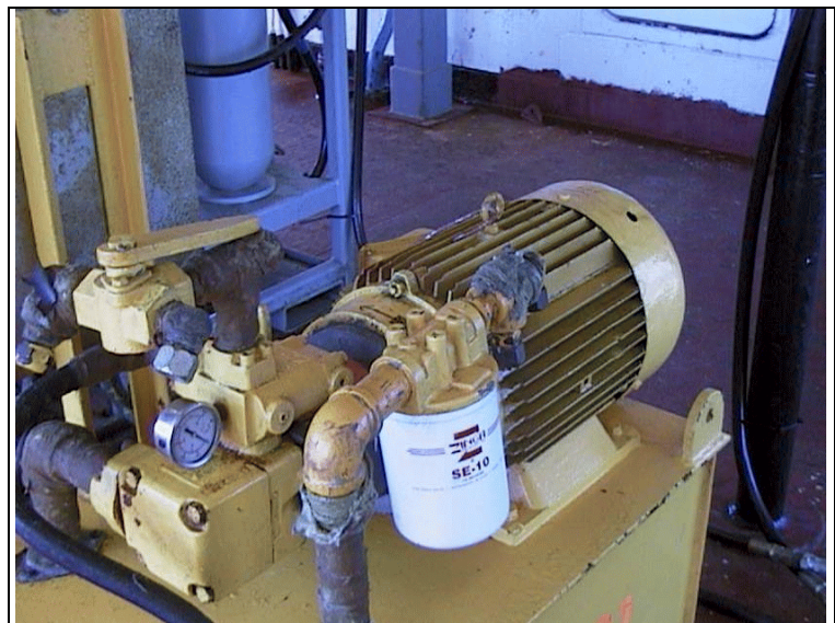
Figure 9 The white filter on the yellow tugger winch decoupled during retrieval of the airgun array necessitating a rapid response from the crew to cleanup the hydraulic oil.
