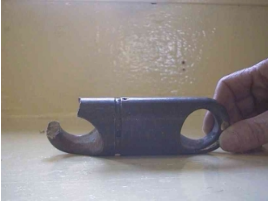
Figure 8. The broken swivel that caused the starboard inboard beam to be towed thwart ship.
