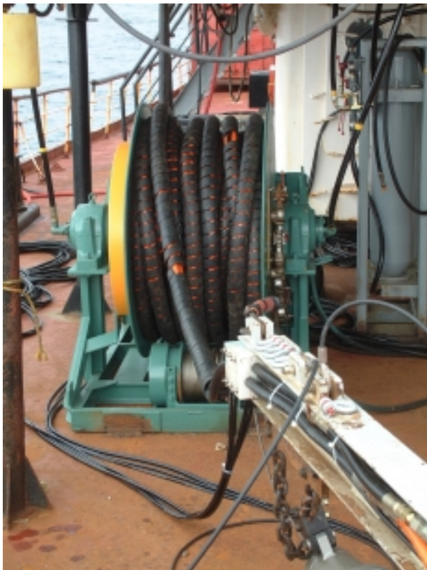
Figure 17. Bundle winch holding the air hoses in preparation for deployment. The smaller winch in front (tugger winch) of the tugger winch holds the wire cables.
