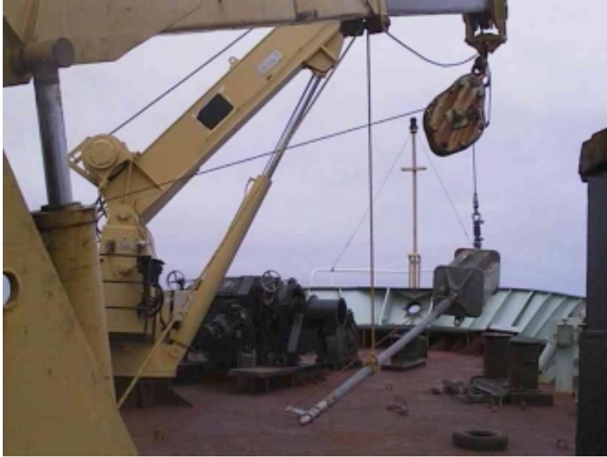
Figure 10. Heat flow probe being lifted by the crane on the fore deck of CCGS Hudson
